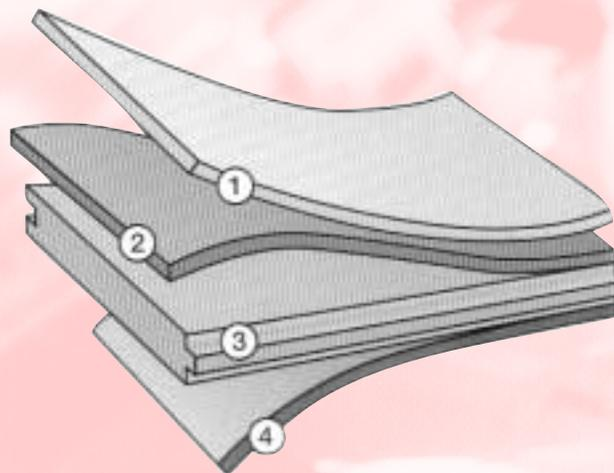
Classen Laminate Flooring is made using direct-pressure laminate technology. The decorative layer\* k along with the wear layer j lies on top of the supporting layer made from high-density fiberboard (HDF) l. The balancing layer m is located beneath the supporting layer. These are floors engineered for a long life.
